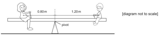
A boy of mass 35 kg sits at one end of the plank with his centre of gravity 1.20 m from the pivot. The see-saw balances when a woman of mass 60 kg sits on the plank on the other side of the pivot. Her centre of gravity is 0.80 m from the pivot.
