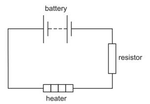
The total resistance of the circuit is  $15\,\Omega$ . In 3.0 minutes,  $180\,J$  of electrical energy is transferred into other forms in the heater.
