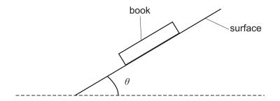
When the angle of tilt  $\theta$  is 20°, the book slides down the slope at a constant speed.
