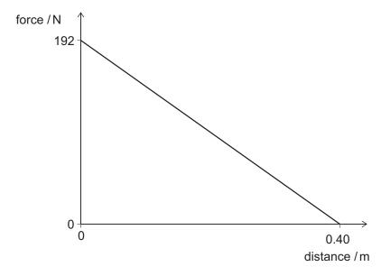
The work done by the force of the bowstring is given by the area under the force-distance graph.
