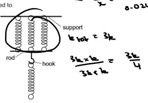
The load of 8.4 N is attached to the bottom of the lower spring.
