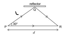
There is a phase difference of  $\pi$  radians between the incident and reflected wave at Q.
