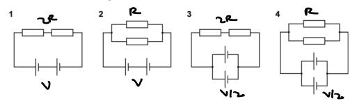
The cells are identical and have no internal resistance. Each cell can supply the same total amount of energy at a constant voltage before becoming exhausted.
