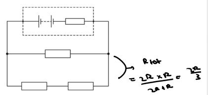
The three identical resistors in the external circuit each have resistance R.
