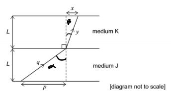
The wave travels a distance q in medium J and a distance y in medium K.
