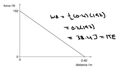
The work done by the force of the bowstring is given by the area under the force-distance graph.
