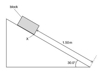
The block is released and it accelerates uniformly down the slope. When X reaches the bottom of the slope, the speed of the block is 2.00 m s<sup>-1</sup>.
