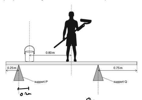
What is the force exerted by support Q on the plank?
